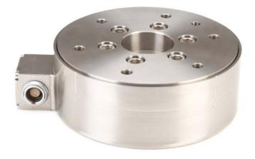
Perry elaborates that ATI's Force/Torque Sensors are largely immune to crosstalk. Load cells typically measure just one or two axes of loading, which can unintentionally react to loads on other axes, resulting in undesirable crosstalk. Six degree of freedom transducers don't have this type of crosstalk problem. Another advantage with the ATI sensors is the availability of
